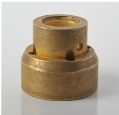
Fig. 3. Used swirl core of the ROsa centrifugal nozzle atomizer
